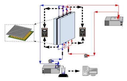
**Figure 14.** Schematic diagram of the experimental setup for the DCMD system of the channels with inserting diagonal carbon-fiber spacers.
