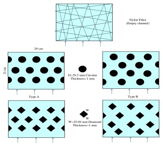
Figure 7. A schematic diagram of three flow channel types.
