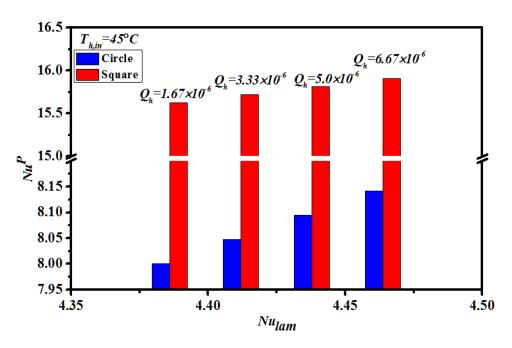
**Figure 10.** Comparisons of theoretical Nusselt numbers for the channels with inserting two geometric shapes and Type A of turbulence promoters.
