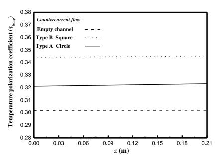
**Figure 13.** Effects of geometric shapes on  $\tau_{temp}$  of countercurrent-flow operations.
