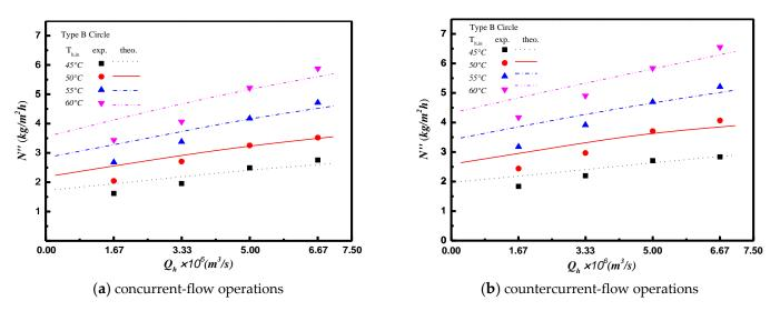
Figure 12. Effects of saline water flow rate and flow pattern on permeate flux for Type B Circle turbulence promoter.
