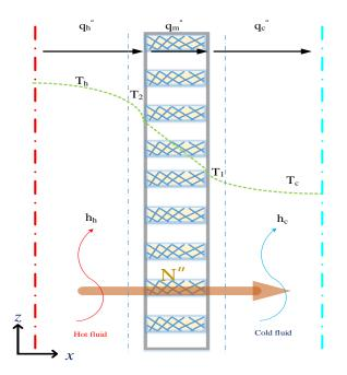
Figure 5. Mass transfer mechanisms and thermal boundary layer in the DCMD module.
