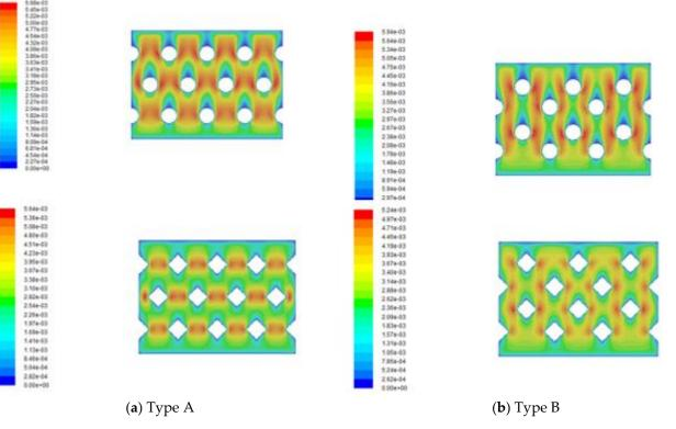
Figure 8. Simulation result of velocity profiles in different arrangements of turbulence promoters.
