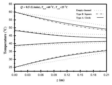
Figure 9. Effect of geometric turbulence promoters on temperature profiles.
