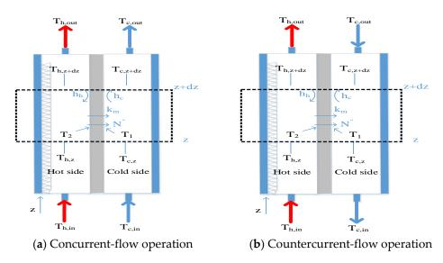
Figure 6. The energy balance made within a finite fluid element (concurrent-flow operations).
