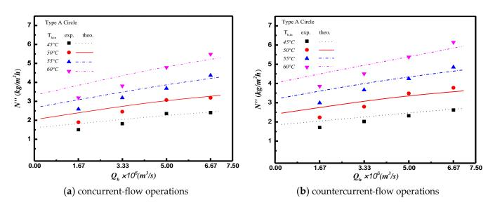
Figure 11. Effects of saline water flow rate and flow pattern on permeate flux for Type A circle turbulence promoter.
