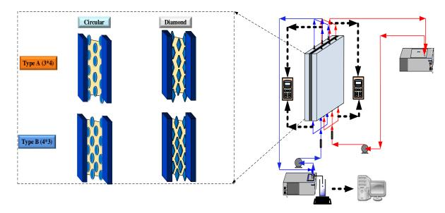
Figure 1. Schematic diagram of the experimental setup for the direct contact membrane distillation (DCMD) system.
