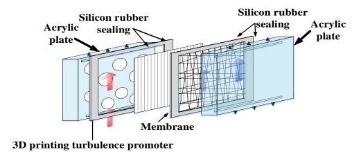
Figure 2. Fabrication structure of the DCMD module.
