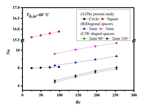
**Figure 15.** Comparisons of theoretical Nusselt numbers of the channels with inserting 3D turbulence promoters and two type of carbon-fiber spacers (countercurrent flow).
